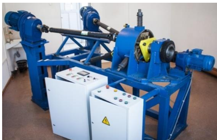
Figure 1 - Radial-shear rolling mill SVP-08
