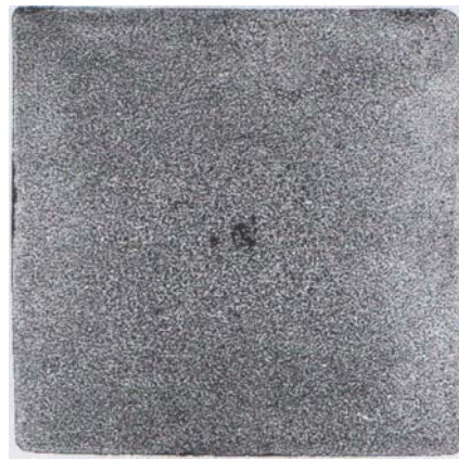
Macrostructure of continuous cast billet blown by nitrogen (A) and mixtures of argon and nitrogen (B) in LHF
